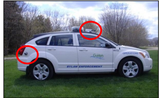
Parking enforcement vehicle with cameras highlighted
