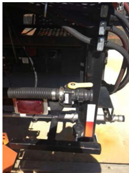
Picture # 2 Fill Valve # 2
